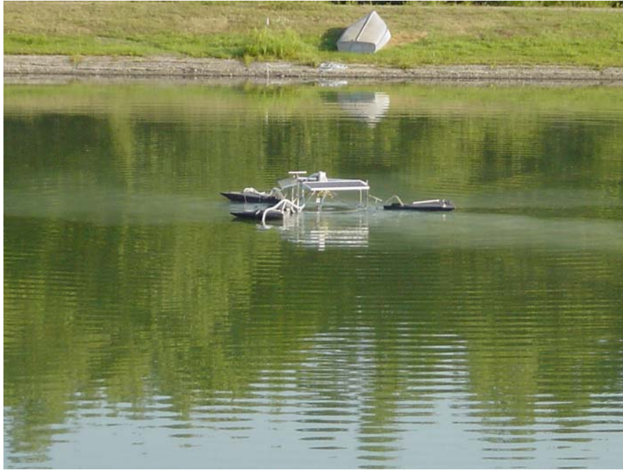
Figure 10 : Circulator, during alum application for Test #2 at Belle Plaine.
