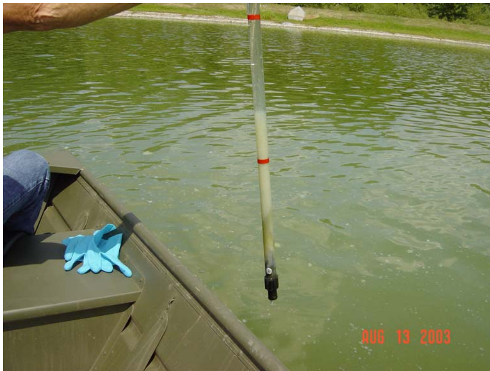
Figure 13 : Sludge judge sample from the bottom of pond near the circulator, during Test #2 at Belle Plaine. The alum floc on the bottom of the pond was approximately 1.25 feet thick.
