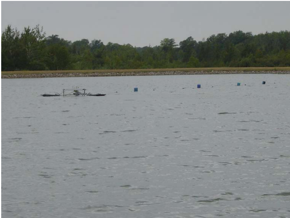
Figure 17 : Alum application during Test #4 at Isle. Additional floats were added to keep the injection hose suspended off the bottom of the pond.
