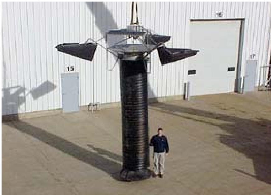
Figure 2 : SolarBee Model SB10000 solar powered circulator. The machine used in the subject tests had an adjustable intake hose length, for 3 to 10 feet deep settings
