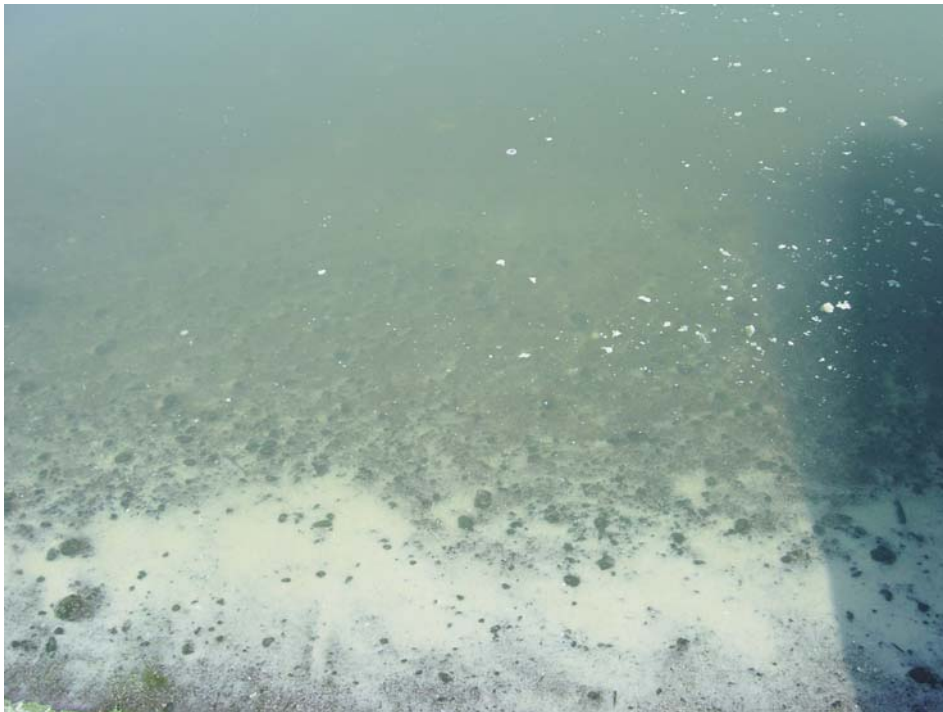
Figure 11 : Alum floc on the bottom of the pond near shore during Test #2 at Belle Plaine. Notice alum floc on pond water surface. The high application rate was a factor in the amount of floc on the bottom and on the water surface.
