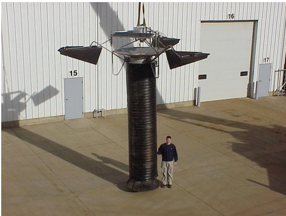
Solar Bee model SB10000 with draft tube
