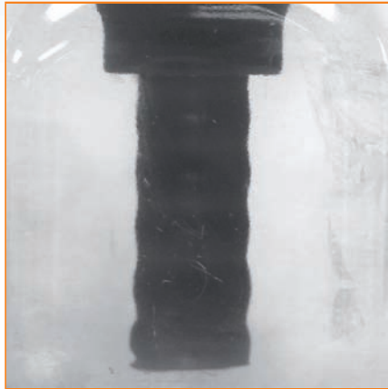
After: inserting the high-performance earth magnet rod assembly into the protective special coated sleeve, all the sludge (magnetite) is retained and trapped on the protective sleeve until a Wash-Down / Rinse-out is performed.
